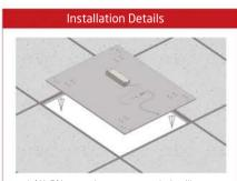
LAY-ON mounting on suspended ceiling
